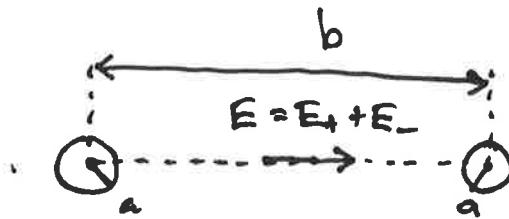
The voltage difference is  $V = - \int_{\text{path}} \bar{E} \cdot d\bar{s}$
