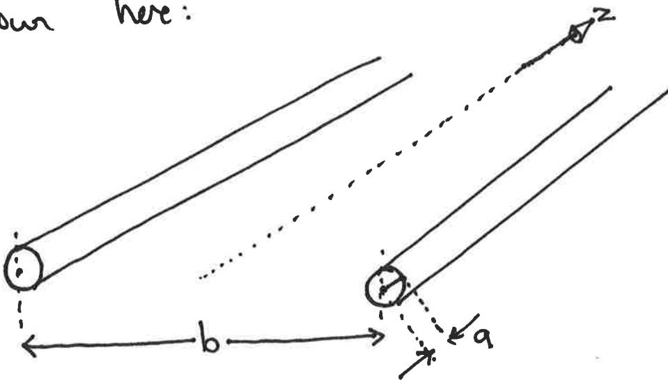
The wires have radius  $a$ . The signal can be represented by voltage and current waves:
