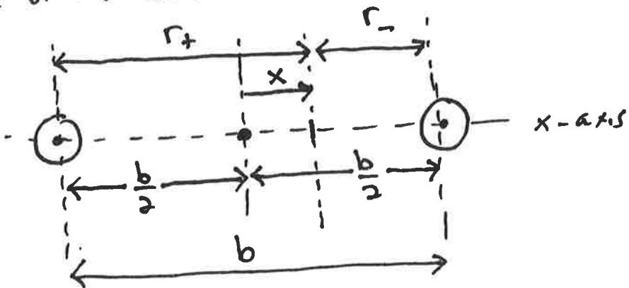
$$r_+ = x + \frac{b}{2} \quad r_- = \frac{b}{2} - x$$
