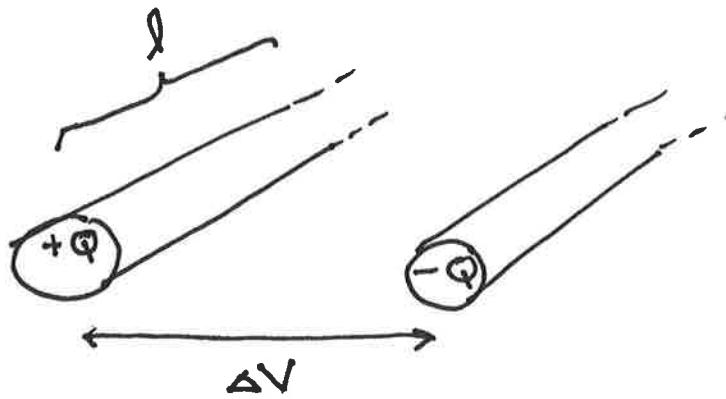
To find the voltage difference  $\Delta V$ , we must integrate the electric field produced by the charges along a line between the wires. The electric field looks like this:
