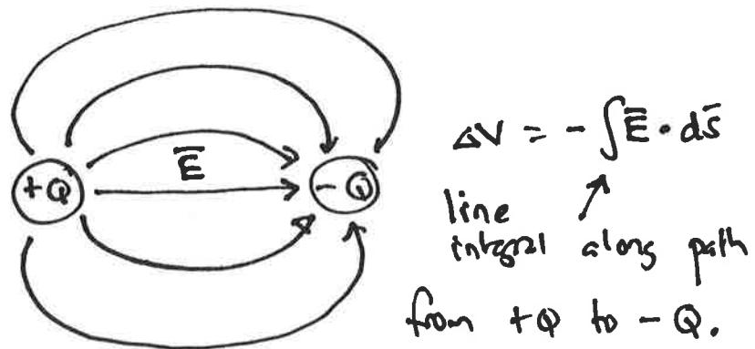
What, though, is the electric field? To find this, we just use Gauss's law to find the field produced by each wire separately and then sum the electric fields. Consider the  $(+)$  wire
